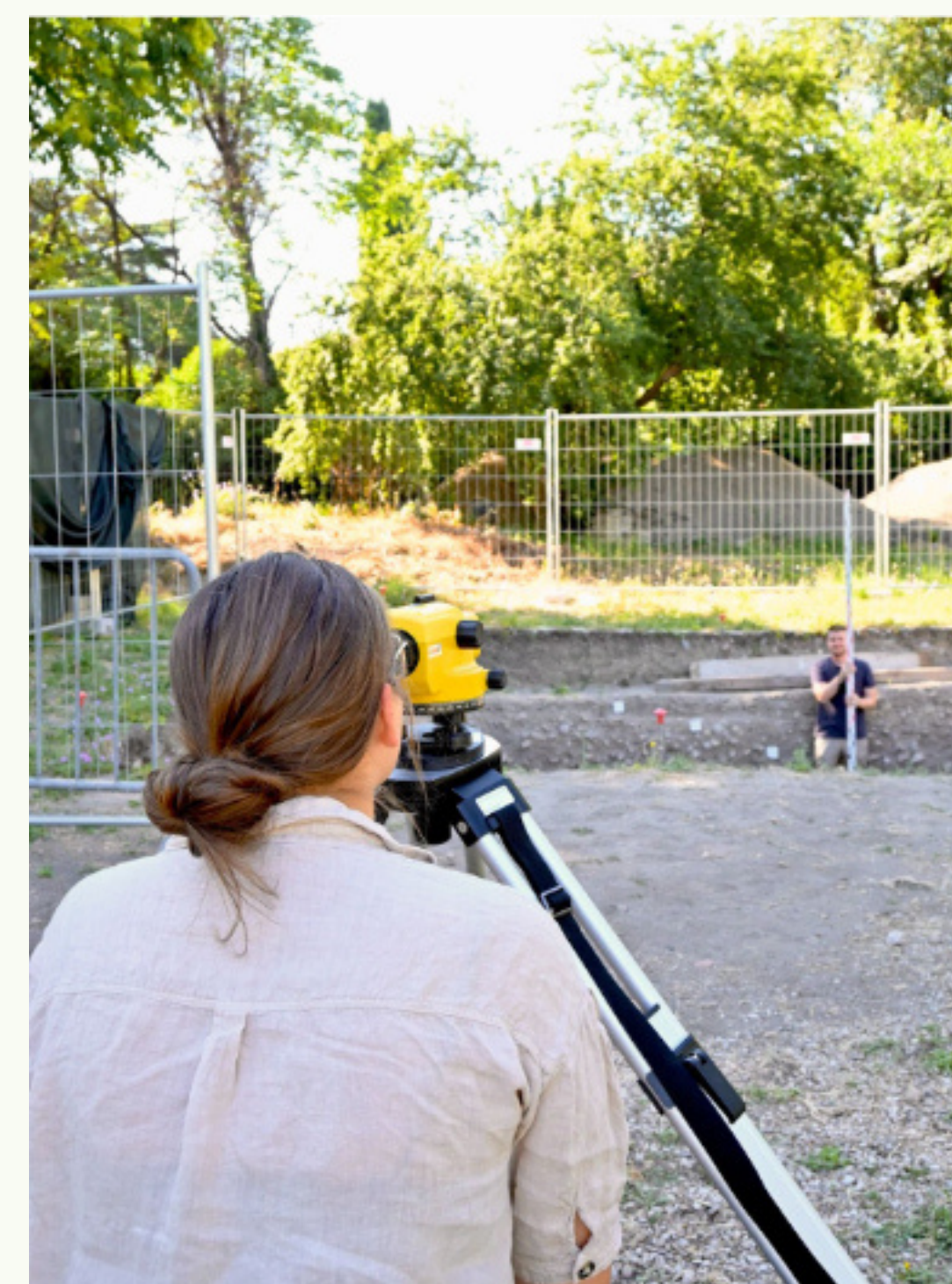
Fig 4: The physical documentation of vertical elevations, using an optical level (foreground) and stadia rod (background).
